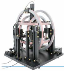
Our magnet unit is developed to provide a very precise threedimensional magnetic field for your DUT - constant or oscillating and in any desired direction in space. The frequency can go up to 150 kHz. If required, you can combine the magnetic excitation with different measures.
