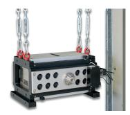
APS 420 with modal stinger (APS 8610 ) and steel cable kit (APS 8612) prepared for free body mode operation
