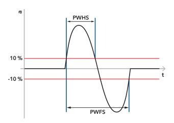
1) PWHS = Pulse Width Half Sine Wave; PWFS = Pulse Width Full Sine Wave
