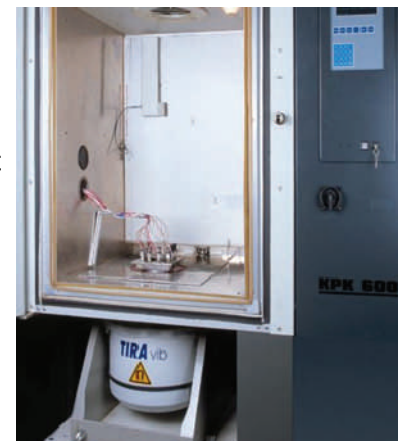
Climatic testing or combined testing of vibration / temperature
