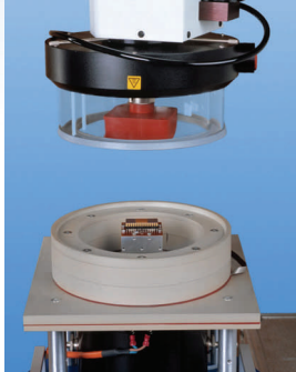
Vibration testing of small modules under ThermoStream®
